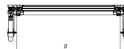
Fig.70 - B-B horizontal cross-section through mcr OSO THERM 75 smoke exhaust window in closed position
